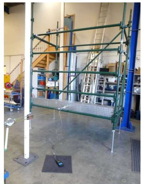
FIG.3 LOAD TEST OF TOEBOARDS
