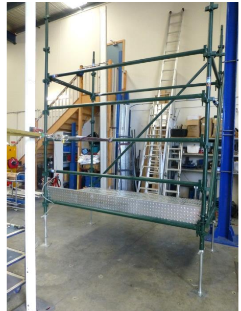
FIG.3 LOAD TEST OF MIDRAIL
